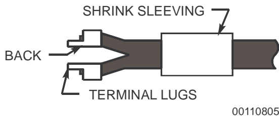
Figure 5 Terminating Braid with Two Lugs
