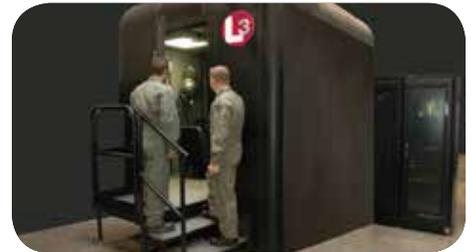
RCTDs are integrated with projected instrument displays, physical fidelity modeling of critical switches, an acoustic seat shaker and a helmet mounted visual display that provides aviators with a 360 degree field-of-regard. Each RCTD configuration simulates specific aircraft radio communications and digital messaging capabilities. Aircraft survivability equipment and weapon systems are modeled for each aircraft and are fully interoperable with the OneSAF threat environment.
